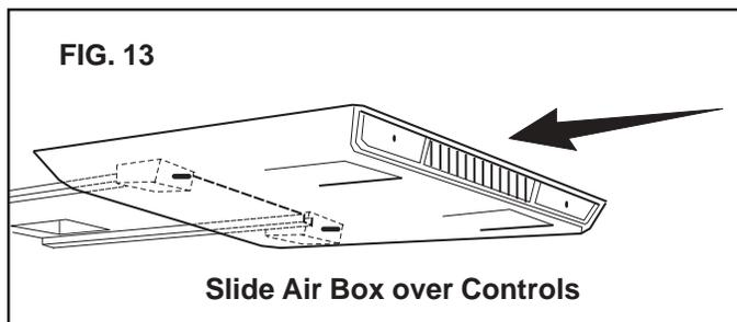
3. Install four screws through legs in air box into the pre-punched holes in the ceiling template.
