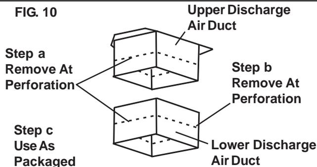
7. Install ceiling template by sliding lower duct over upper duct. See FIG. 11.
