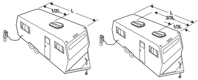
It is preferred that the air conditioner be installed on a relatively **flat and level** roof section measured with the RV parked on a level surface.
